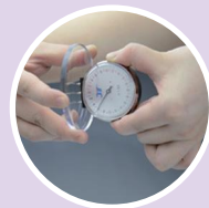
3. 垂直测量反面度数 Measure the reverse side vertically
