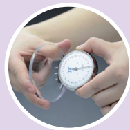
2. 垂直测量正面度数 Measure the front degree vertically
